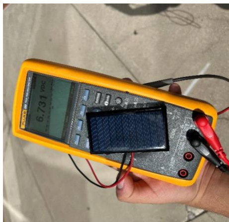
Figure 23 - Solar Panel voltage testing
